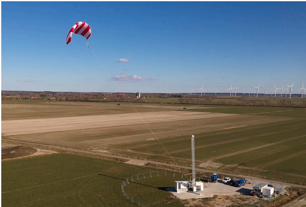
Fig. 2. The researched test site featured a ground-gen airborne wind energy system with a soft-wing kite. In the background, one of the many nearby wind farms is visible (Courtesy of the SkySails Group).
