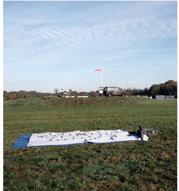
Figure 2: Acoustic array used during the measurement campaign
