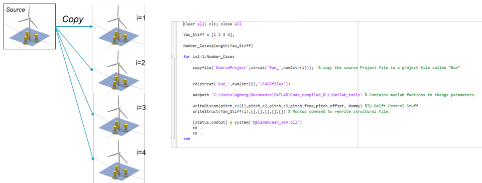
Figure D.1: Graphical representation of the desired workflow using QBlade as .dll within Matlab. The Matlab code included is only for illustrative purposes.
