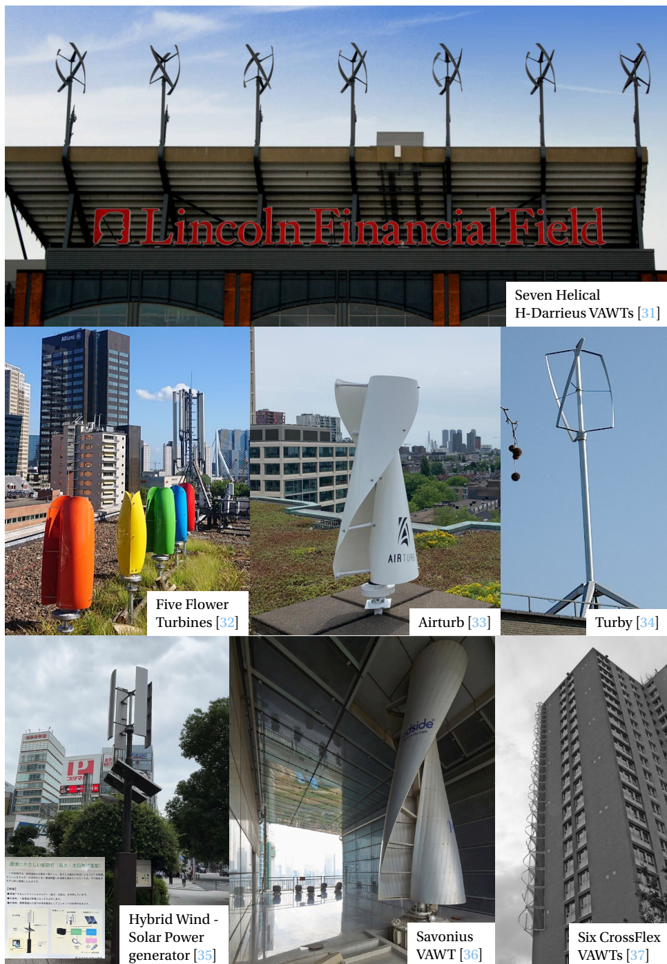
Figure 1.2: Overview of vertical-axis wind turbines (VAWTs) in urban environments. Seven of the fourteen H-Darrieus VAWTs with helical blades installed on the Lincoln Financial Field stadium in Philadelphia (USA) [31], five 100 W Flower Turbines [32] installed on a rooftop in Rotterdam (NL) (Photo by M. van den Broek), the 300 W Airturb wind turbine designed by Airturb [33], the 2.5 kW Turby designed by Delft University of Technology [34], the Hybrid Wind-Solar Power Generator CPH 200 W [35] installed in the street of Tokyo (JP) (Photo by L. Brandetti), one of the four Savonius VAWTs installed in the Pearl River Tower in Guangzhou (CN) [36] and the six CrossFlex VAWTs installed on the Newbery Tower in Glasgow (UK) [37].
