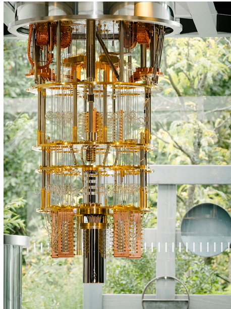
(b) IBM cryostat hosting a 50-qubit chip (50Q system) from 2017 with stacks of circulators/isolators at the bottom left and right. Picture taken from IBM Quantum Blog “The Future is Quantum” (Nov. 2017).
