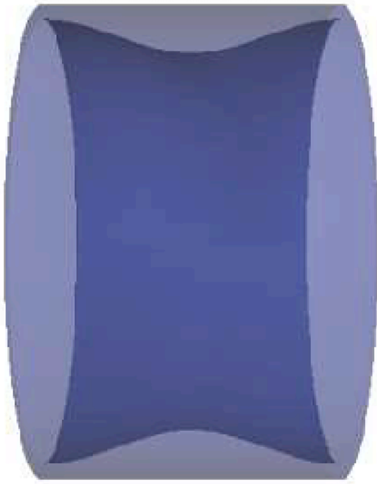
Fig. 5. Geometry for the annulus flow with a fixed wavy inner wall.
