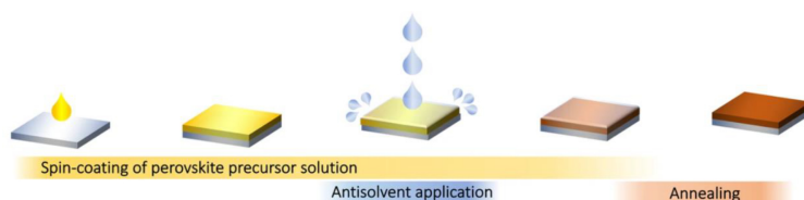
Figure 1.4: Schematic representation of the perovskite film fabrication process using an antisolvent, adapted from ref 28 .
