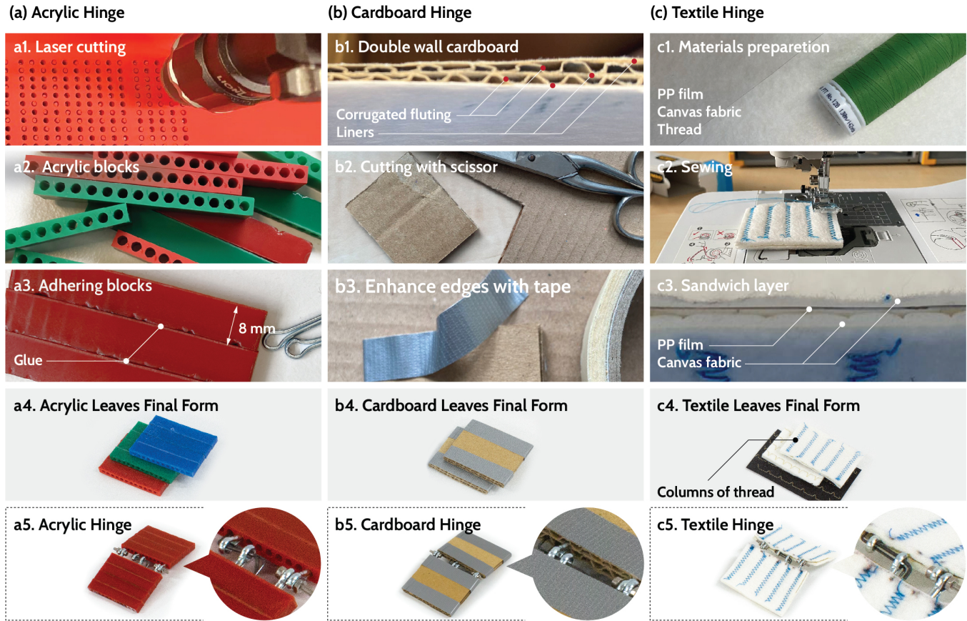
Figure 4: Hinge leaves based on three types of materials: configuration process and their structures. (a) Acrylic hinge leaves: acrylic blocks are manufactured by laser cutting, and then each four blocks are glued and combined together as a hinge leaf. (b) Cardboard hinge leaves: they are made from cardboard package box. (c) Textile hinge leaves: the sandwich structure leaves include two layers of fabric and one layer of PP film in the middle. Note that there is no limit of the type of fabric, but 2-3 mm thickness fabric is recommended. (a5), (b5) and (c5) show three types of hinge and their connection details. More details are explained in the Hinge Construction part of section 4.
