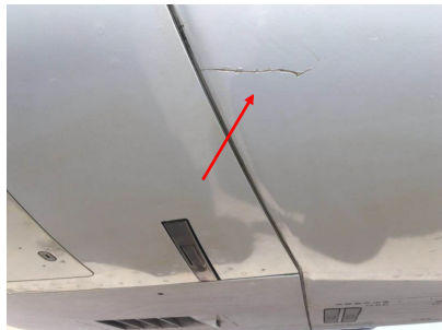
Figure 1.4.: Crack size in the fuselage. This picture is from [68].
