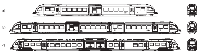
Fig. 5. Graphical representation of Stadler's multiple unit vehicles employed on the Northern lines: (a) GTW 2/6, (b) GTW 2/8, and (c) WINK [17,102].
