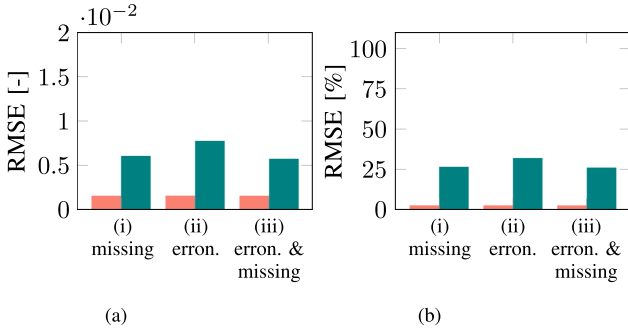
Fig. 9. Comparison of RMSE for the estimation of (a) voltage level and (b) line loading between WLS (■) and DSS 2 (■) in the 70-bus network considering (i) missing voltage measurement, (ii) erroneous voltage measurement and erroneous active power flow measurements, and (iii) missing voltage measurement and erroneous voltage measurements.
