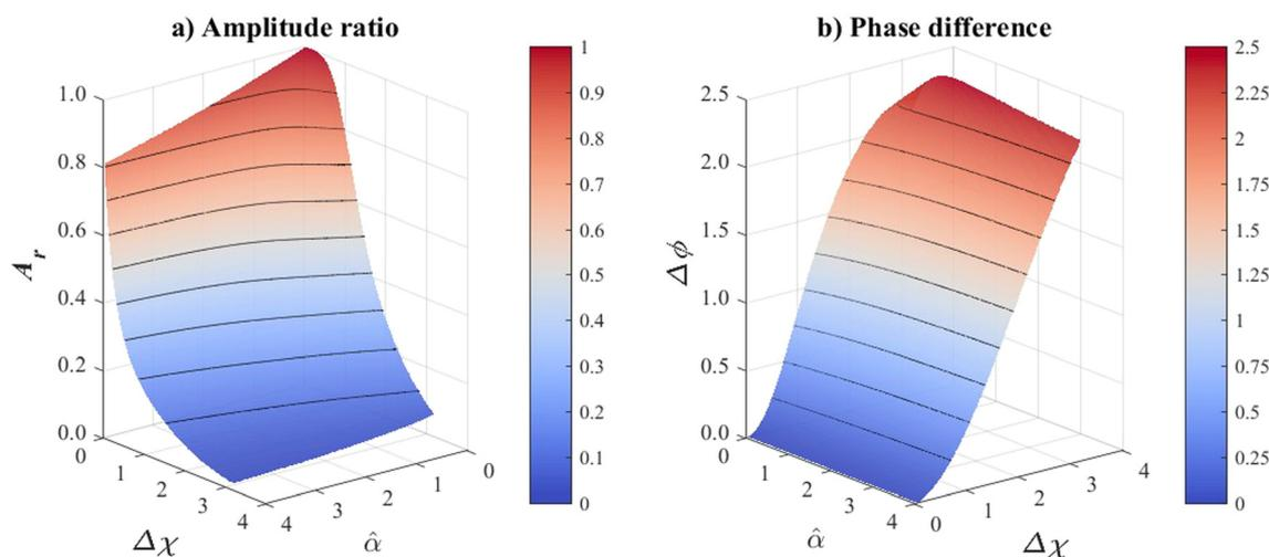
Fig. 3 Relationships between the nondimensional parameters,  $\hat{\alpha}$  and  $\Delta\chi$ , of the 1D diffusion heat equation and the harmonic features, (a) amplitude ratio and (b) phase difference.
