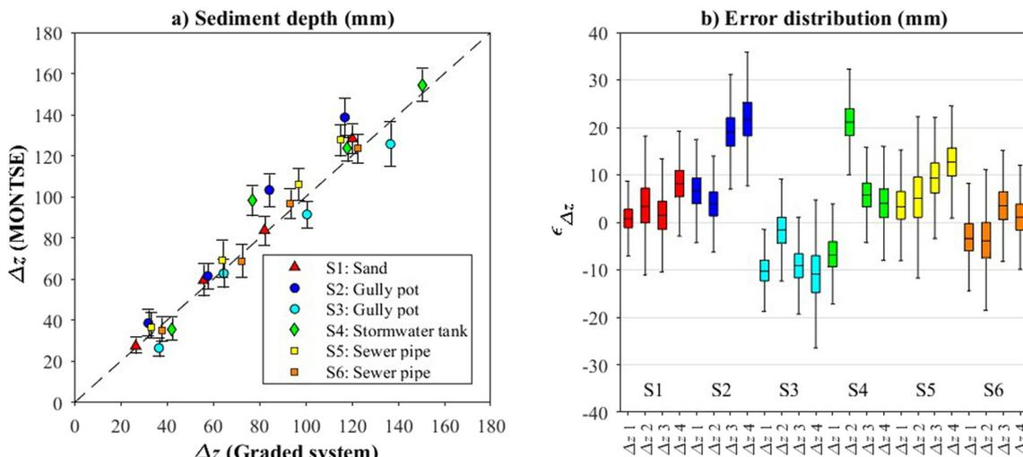
**Fig. 6** (a) Comparison of the sediment depths estimated by the temperature-based system and visual measurements obtained by the measuring tapes. The vertical error bars represent the coverage interval at a confidence level of 95% computed by Monte Carlo simulations. (b) Absolute error distribution of the sediment depths considering the six sediment samples (S1 to S6) and the four depth steps ( $\Delta z_1$  to  $\Delta z_4$ ).
