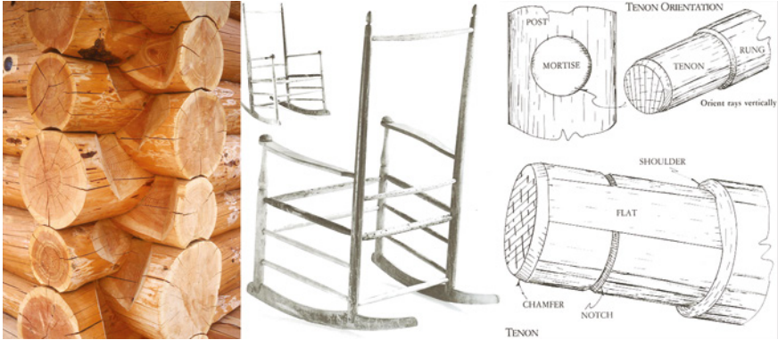
FIGURE 7 Examples of shrink-fit-joints. (Left) The “shrink-to-fit” notch, or Beckedorf Butterfly joint on a log home from Lloyd Beckedorf of Moose Mountain Log Homes (Chambers 2006). (Middle) Shaker rocker chair joined by shrink-to-fit tenon-and-mortise joints ((Alexander 1978). (Right) Details to enhance friction-fit of greenwood shrink-to-fit mortise-and-tenon joints (Alexander 1978)
