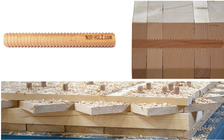
FIGURE 15 (Top left) Threaded beech dowels used in the NurHolz system. (Top right) Cut section of a NurHolz panel showing form- and friction fit of the dowels in the lamellae. (Bottom) DCLT panel production with alternating layer setup and screwed in dowels. All illustrations by ROMBACH Bauholz + Abbund
