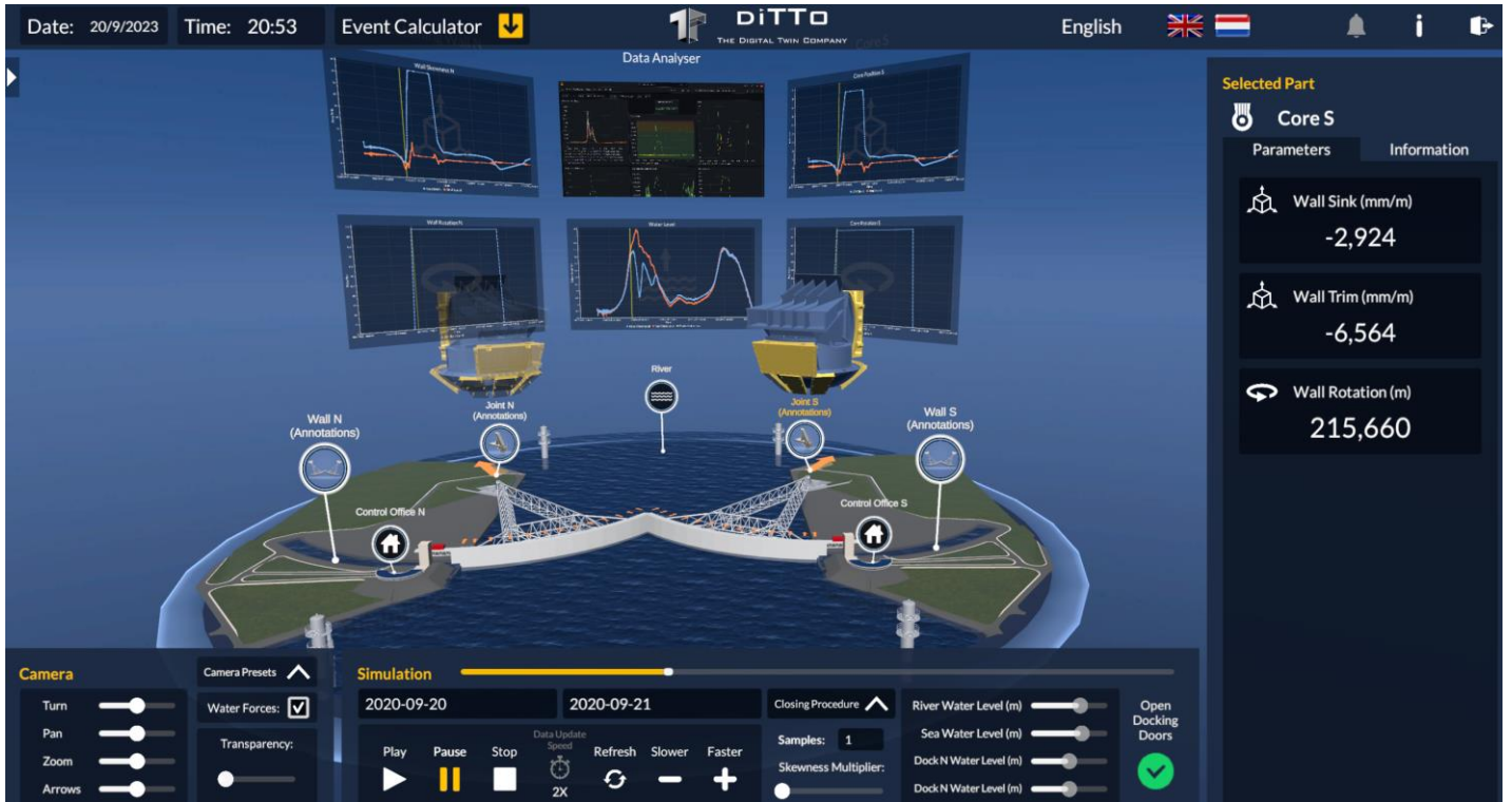
Figure 4: A visualization of the digital twin prototype. It shows the animation of the barrier closing for the actual 2020 test closure (centre), control panels for the simulation or replay of the closure (lower panel), clickable panels for data visualization and further data analysis including water levels, barrier position, pump data and status of valves (top panels) and 'live' values of the animated parameters including the option to search for more information (right side)
