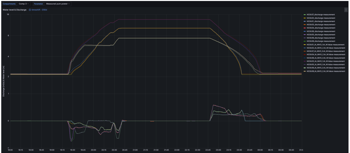
Figure 51: An example of measured water levels in the compartments of the retaining walls during closure of the Maeslant barrier (top graph set). The in- and outflow discharge (bottom graph set) in the compartments is a calculated parameter based on the measured water levels in the time and the dimensions of the compartments.
