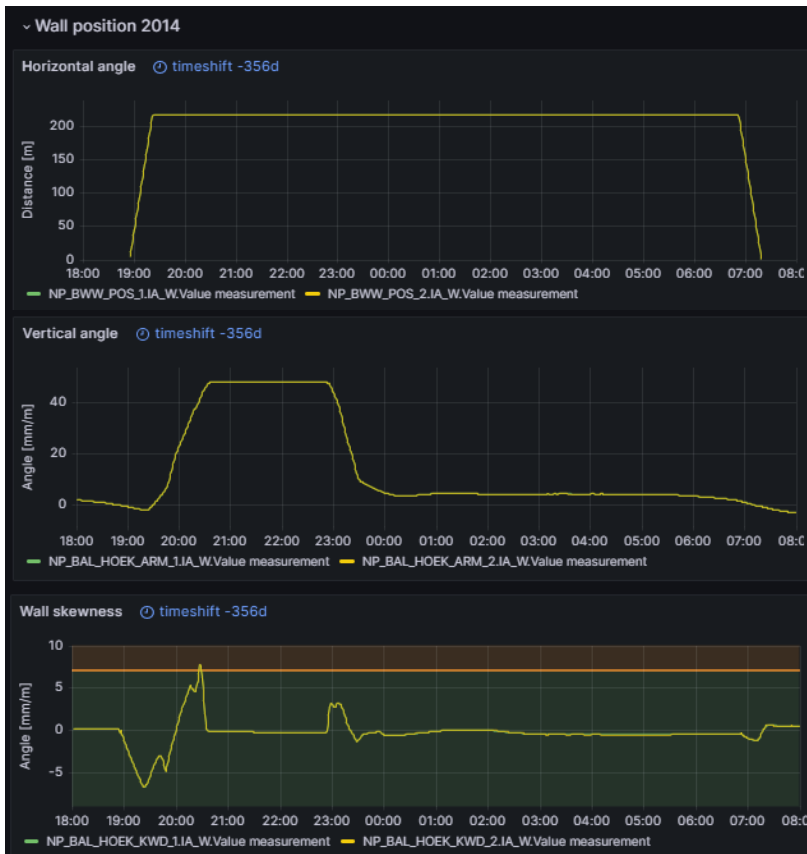
Figure 49: An example of measured values during a closure of the barrier. In this case the horizontal movement (top graph), sink angle (middle graph) and skewness (bottom graph) of the retain wall is visualized
