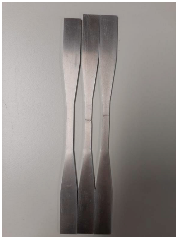
Fig. 4. Yield test structure a) applying tension to a dog-bone aluminum using Instron machine and attached LVDT to measure the strain. B) Comparing two broken specimens with a true specimen
