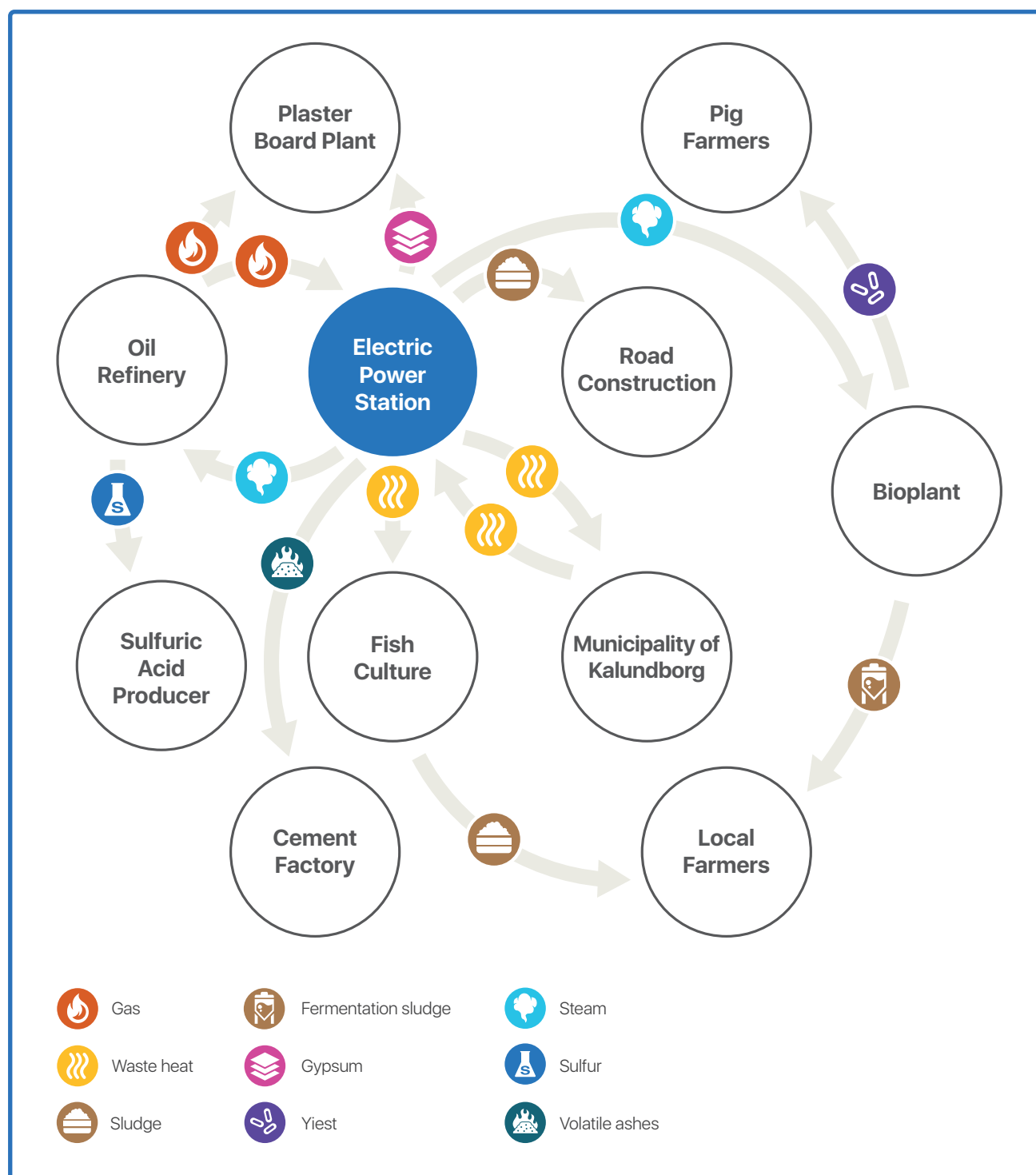
Figure 2 The flows of material, energy and water in ecosystems (previous page) are mimicked in an industrial symbiosis between firms that exchange waste as a resource (current page). Source: Lao et al. (2020) and Kalundborg Symbiosis
