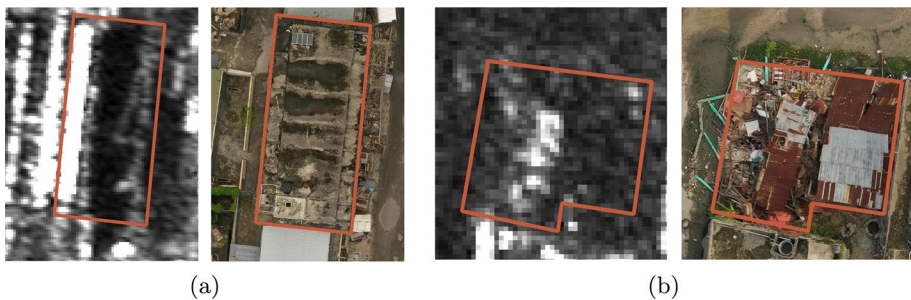
Fig. 1 Building appearance in VHR SAR imagery and a drone orthophoto: a an intact building, and b a collapsed structure. The VHR SAR data is sourced from Capella imagery acquired over Les Cayes, Haiti (©2021 Capella Space, all rights reserved)
