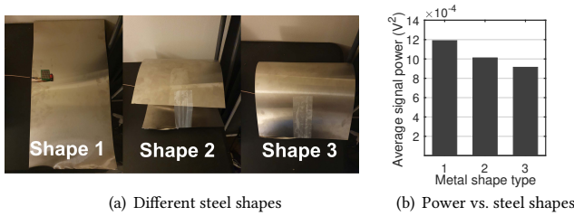
Figure 8: Power vs. steel shape: (a) Different steel shapes as: flattened (type 1), curved (type 2) and closed cycle (type 3); (b) Average power of the received leaked energy from coils with different surrounding steel shapes.
