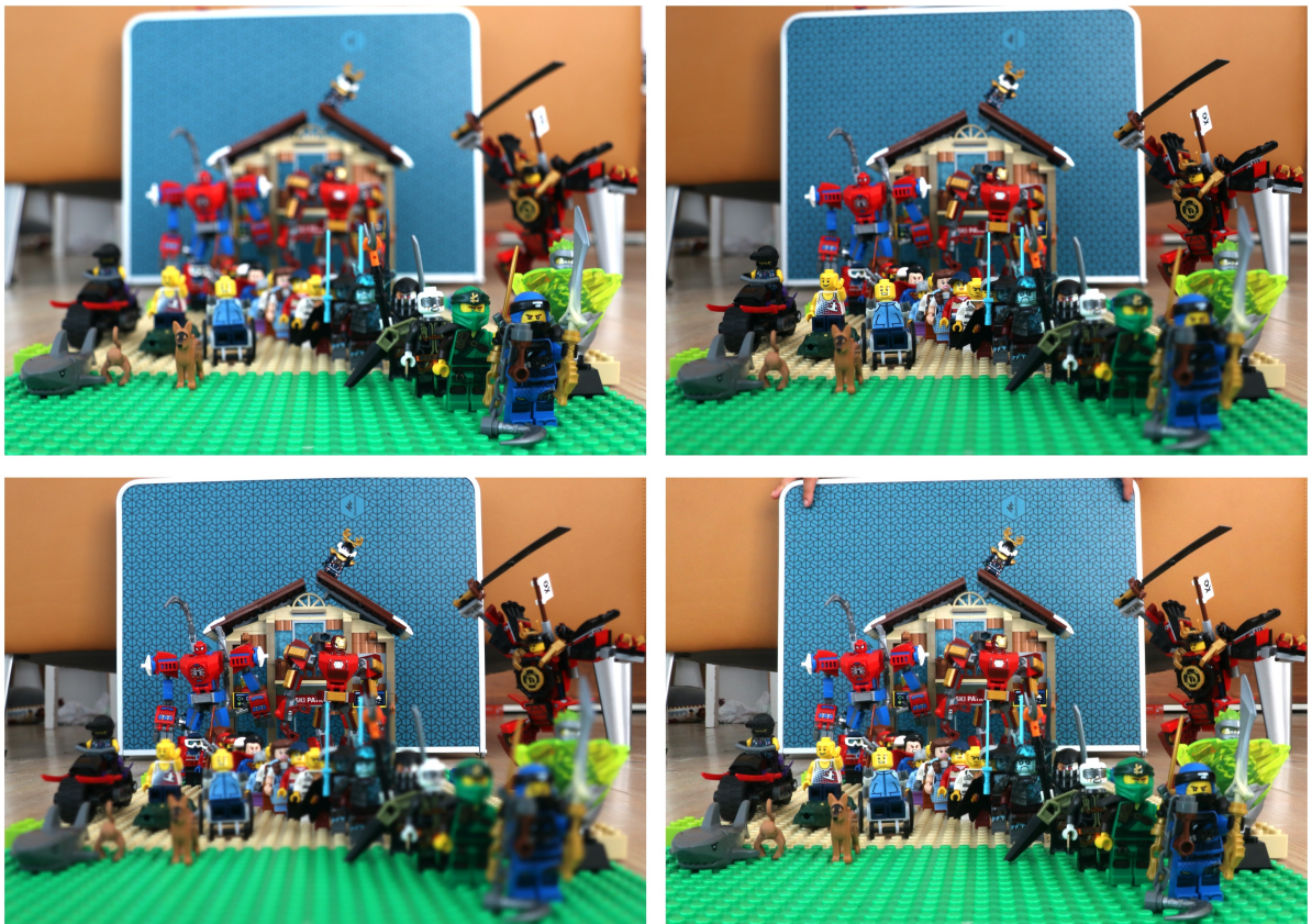
Figure 3.4: Four images taken with different diaphragm and different focal plane. The image on bottom right is taken with a small diaphragm and the entire image appears clear (photos taken by Aurèle J.L. ADAM / CC BY-SA).
