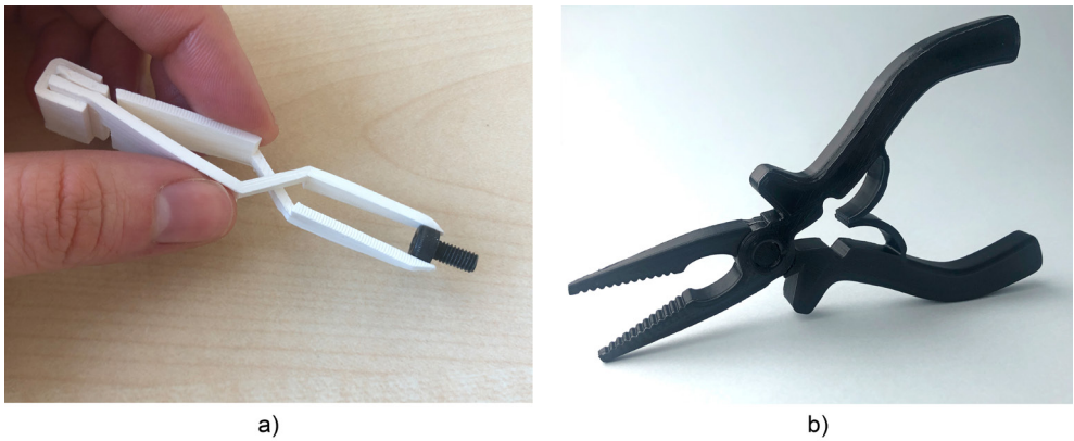
Figure 3.5: Examples of leaf springs. a) Crossed leaf springs applied in self-closing tweezers, based on [53]. b) Leaf springs applied in self-opening pliers, based on [52].
