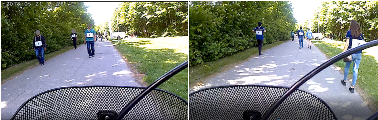
Fig. 3. Meeting (left picture) and Passing (right picture) conditions seen from the action camera placed on the e-bike representing the rider's perspective.
