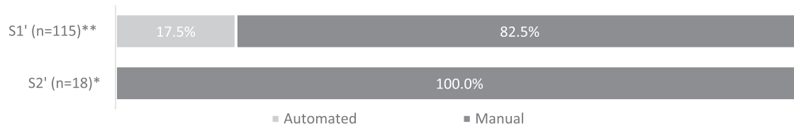
Figure 5. Solar shading device control types encountered in sample S1 (top) and subsample S2 (bottom). Source of data: *On-site verification; ** Survey.
