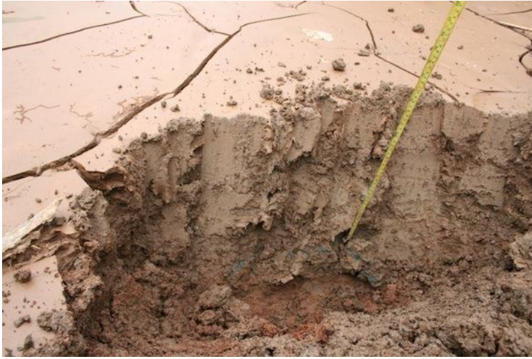
Figure 2.11 Dye was found about 30 cm from the sediment surface.
