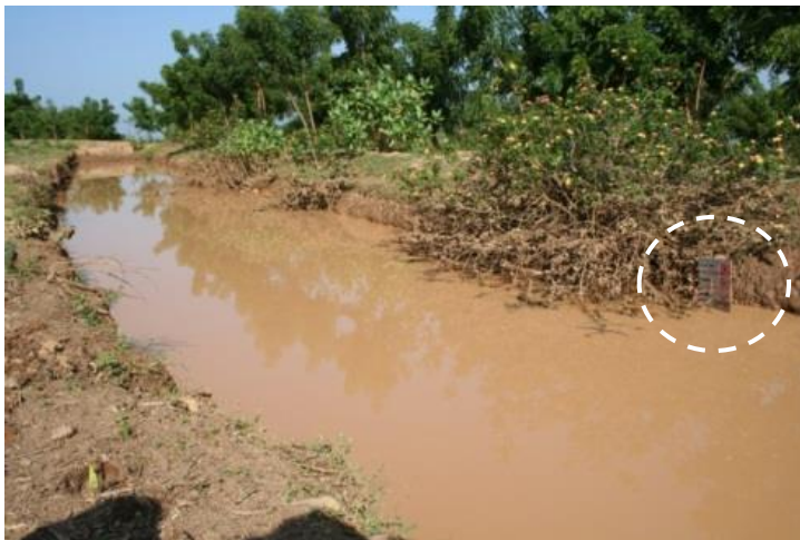
Figure 2.2 A Casella tipping bucket, next to it a manual rain gauge and a locally made evaporation pan at the roof of the temple (upper) and ponded Trench 1 with a scale of the depth in circle (bottom).
