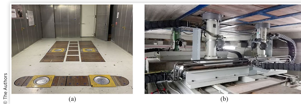
FIGURE 6 (a) Semi-anechoic chamber in which vehicle is placed on the 4-poster test rig; (b) room below the floor of the semi-anechoic chamber housing the actuators.
