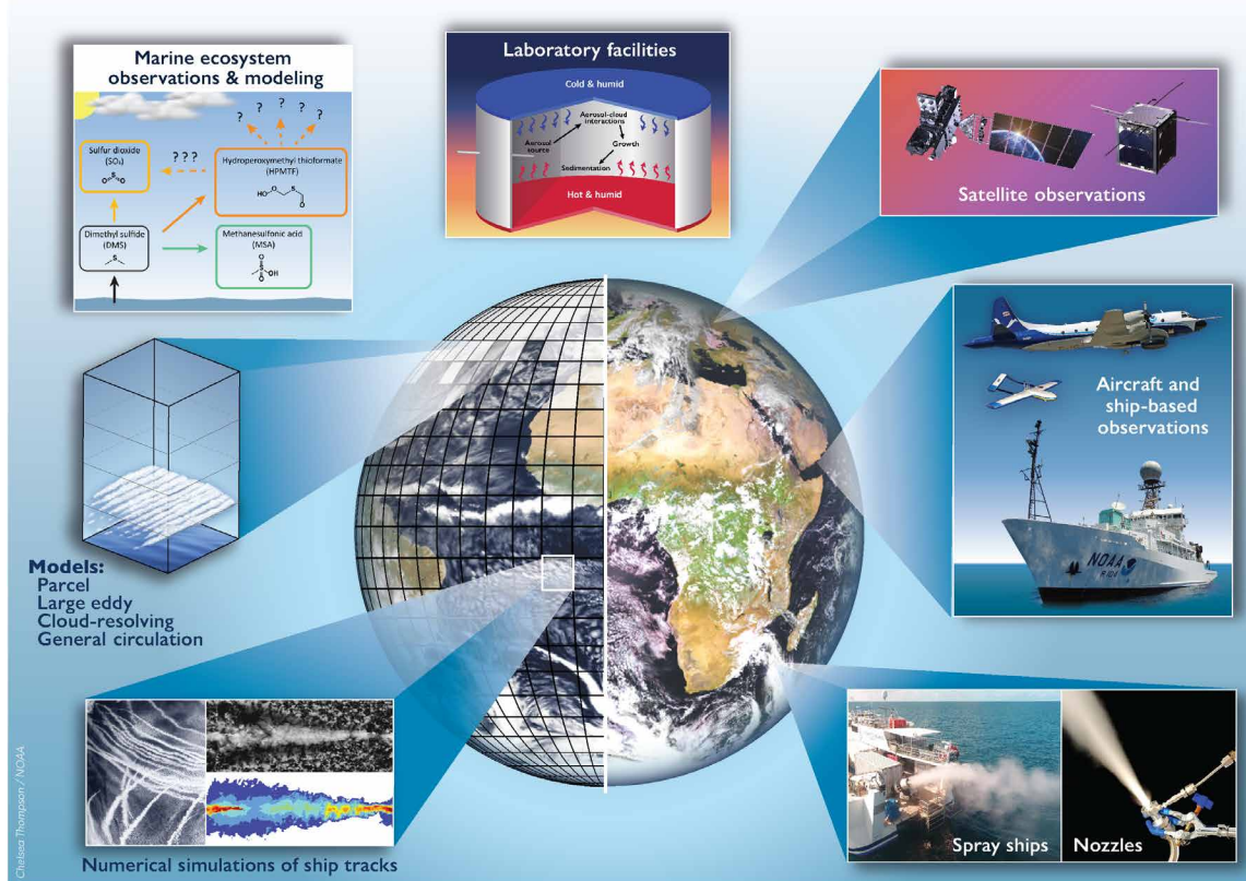
Fig. 4. An integrated approach to a marine cloud brightening research program comprising laboratory facilities, field experiments, and modeling. Laboratory facilities such as cloud chambers together with observations at a range of scales will help improve the representation of physical processes in models. Parcel models, large eddy models, and cloud-resolving models will inform the global model activities to improve the reliability of regional climate responses. The Earth view image is courtesy of the European Organisation for the Exploitation of Meteorological Satellites (EUMETSAT).
