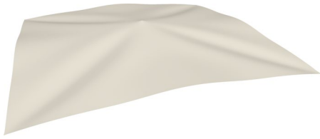
Fig. 13 Deformed surface from the benchmark presented in Fig. 12. The result is the last solution from the adaptive meshing routine with deformation norm goal-functional of which the results are presented in Fig. 14
