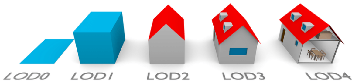
Figure 1. Levels of Detail for buildings according to CityGML v. 2.0. Image source: Biljecki et al. (2016)
