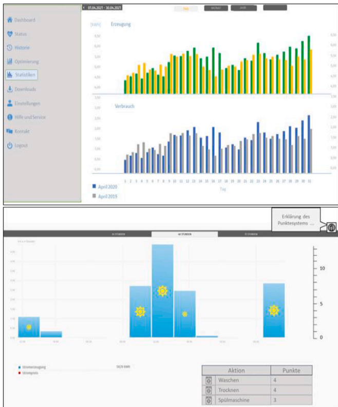
Fig. 3. Intervention 2 for the PV- and EV-group providing benchmark of previous and current self-consumption (top) and forecast of PV-generation with recommendations for actions (bottom) to stimulate consumption shifts or additional consumption during PV-generation by the participants, as presented to the participants and thus, in German language, see supplementary material for further information.
