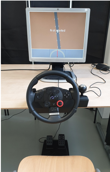
Figure 5.2: The experimental setup as seen from the view of one participant. The participant sees a top-down view of the vehicle they can control with the gas and brake pedal. The steering wheel provides vibration feedback if the participant deviates from the designated velocity. Visual velocity feedback is provided through the speed dial in the lower part of the screen.
