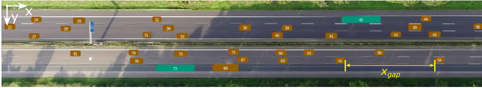
Figure 2.4: An example frame of the HighD dataset [25] as visualized using TraViA [28]. The frame includes a stretch of a highway in Germany, where vehicles drive on the right side of the road and where, in some of the cases, there are no legal speed limits. The orange shapes represent regular cars, the green shapes are trucks. All vehicles have a vehicle-ID shown in white. The white arrows display the coordinate frame and the yellow marking shows a visualization of the gap between two vehicles as used in the metrics for step 3 of the validation workflow.
