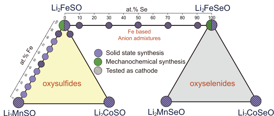
Fig. 3. Schematic illustration of the experimentally reported Li-ion AP cathode materials with different TMs and Chs to date and corresponding synthesis route. The two triangles refer to S- and Se-based compounds, respectively, and the vertices indicate TM end-members. The sidelines correspond to the atomic percentage of each TM or Ch .
