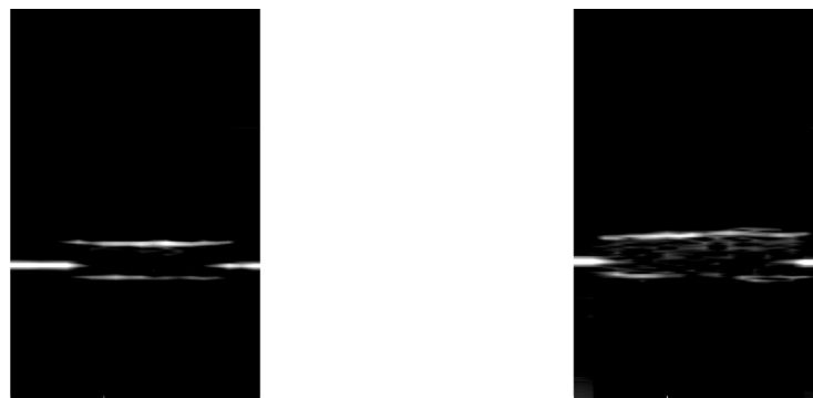
Fig. F.1. OCT images obtained for the analysis of the width of the PC 1-layer printed with the standard (left) and the optimized (right) nozzles at 5 \text{ mm}^3/\text{s} .
