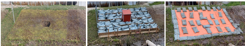
Figure 2.8: (left) Reference case with damage, (middle) plate and (right) sheet Flood Proof Holland
