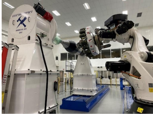
Figure 14. Test article being built on the automated fiber placement robot.
