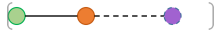
Fig. 6. The case of a node of interest as the first node and at a known position with only one other node, which is at an unknown position, but at the maximum operating conditions.
