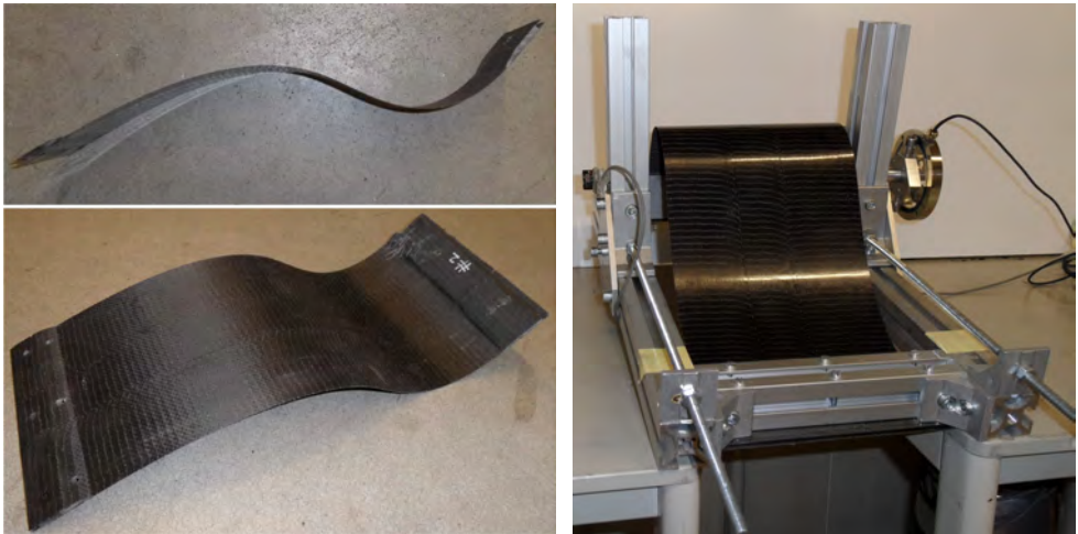
Figure 5.4: (a) Pictures of the carbon leaf spring. (b) Picture of the test setup. On the left hand side the potentiometer is connected with the rotation axis, while on the right hand side the torque-sensor is attached. The rotation is applied to the system by manually turning the outer ring of the torque-sensor. On the bottom the studs with the tensioning nuts are visible.
