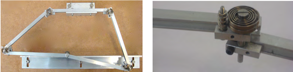
Figure 9.8: (a) Picture of the prototype and (b) detail of a torsion spring at the connection of two links.
