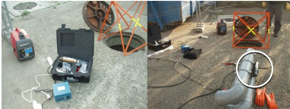
Figure 2. Material used for field experiments in Lyon. Left: sonar equipment; right: the floating El Torpedo with the attached sonar probe (in the middle of the white circle).
