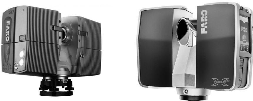
Figure 3: Two models of scanners; FARO Photon 120 (left), FARO Focus 3D X130 (right)
