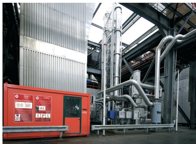
Figure 2. TNO CO 2 capture pilot plant at the Maasvlakte power plant in the Netherlands.
