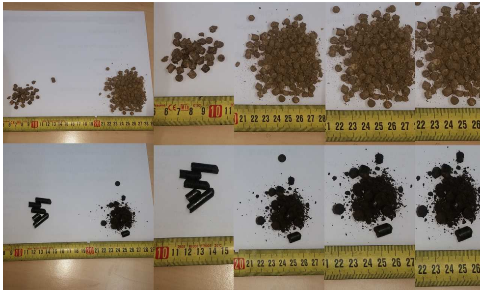
Figure 6.10. Particle size reduction due to feeding system; from right to left Topell black and Topell white.
