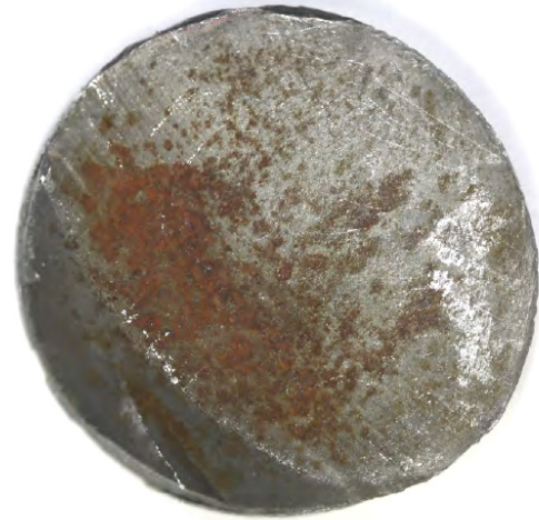
FIGURE 4 - Glass insulator pin fatigue fracture surface
