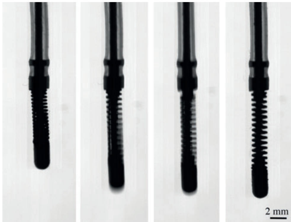
Figure 8.12— Example of a HSV image sequence of the indenter of Pulze . Based on the image sequences, an average indenter velocity of 0.95 \pm 0.15 m/s was derived. The time between frames is 1 ms.
