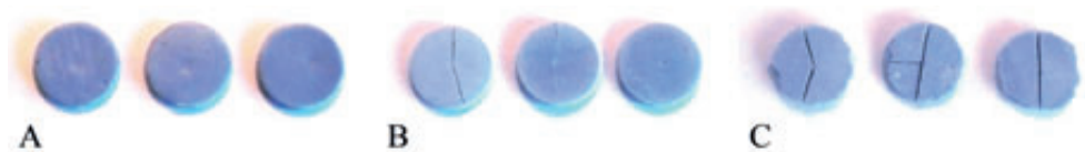
Figure 7.14— Typical Proximal Cap Models after Striking the Indenter Multiple Times Onto Them. The illustrated proximal cap models were struck with the spherical indenter tip shape, on (A) the ductile model (10 strikes on all of the models), (B) the reference model (from left to right: 4, 5, and 10 strikes), and (C) the brittle model (from left to right: 3, 3, and 2 strikes).
