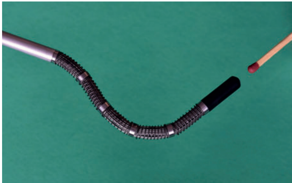
Figure 3.4— Multisteerable Tip of Multiflex . The match is illustrated for scale purposes.
