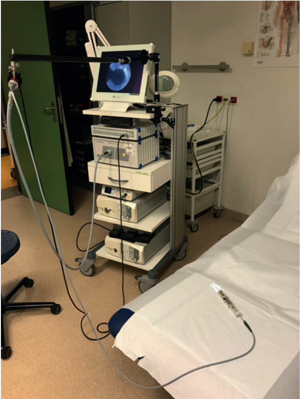
Figure 13.16— Clinical Experimental Facility at University Medical Center (Utrecht, the Netherlands). The experimental facility consisted of the biopsy needle integrated with the micro-endoscope connected to the imaging equipment.
