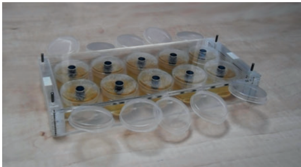
Figure 7.A1— The Mold for Creating the Environment Models. The mold consists of laser-cut disks in between which 10 circular containers can be placed. The lid of the mold, in which several rods are placed, creates the notches.
