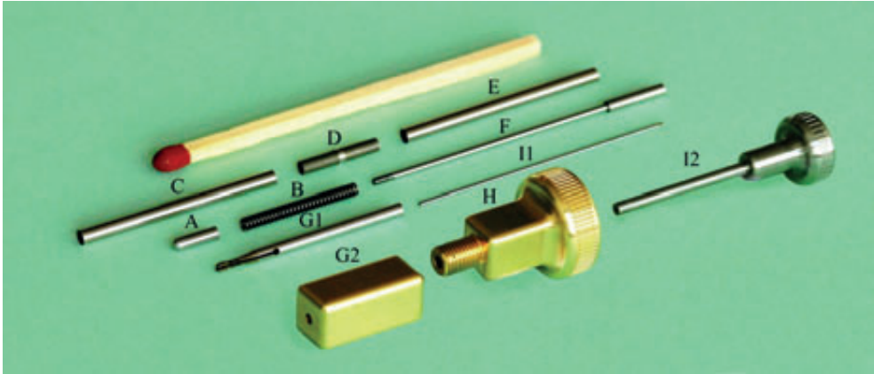
Figure 7.4— Prototype Tip Design and Control Interface. Letter indications: (A) Indenter, (B) Compression spring, (C) Capillary tube front, (D) Position block, (E) Capillary tube back, (F) Indenter stop, (G1) Gripper reload mechanism, (G2) Square sliding bearing connected to the gripper, (H) Handgrip gripper, (I1) Core reload mechanism, and (I2) Handgrip core. The match is shown for scale purposes.
