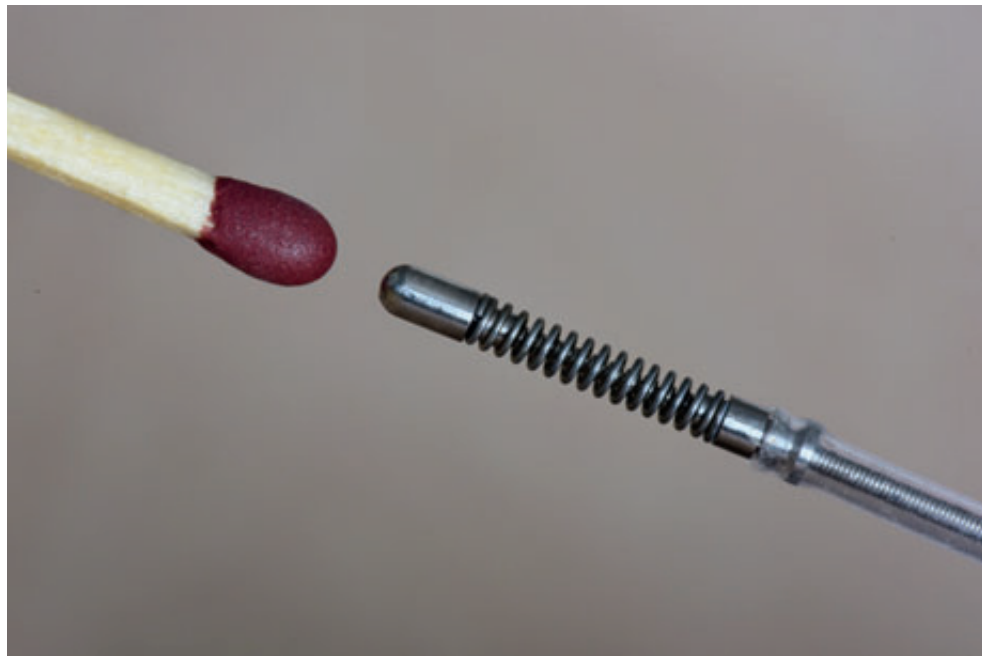
Figure 8.8— Assembled Pulze catheter tip with match for scale reference.
