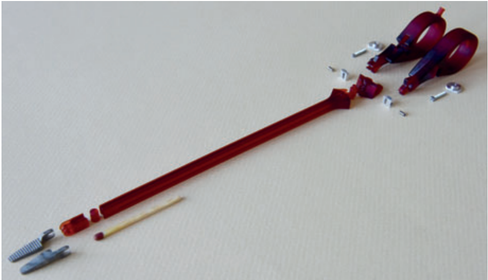
Figure 4.7— Exploded View of the Final Prototype. The final design consists of the two titanium movable tip jaws, joint 1 to move the tip sideways (left-right) with curve angles of \pm 65^\circ , joint 2 to move the tip up and downwards with curve angles of \pm 90^\circ , a rectangular 5 mm shaft to guide the steering ribbons and electrode cables towards the handle, 2 ring handle parts to open and close the tip jaws, 2 tension mechanisms to tension the electrode cables (consisting of a titanium tension bolt and ring; situated in the handle) and steering ribbons (consisting of a stainless steel rectangular box, a stainless steel tension plate and stainless steel M2 set screw; situated in the mirrored joint 1), 2 \text{\O}0.45 mm electrode cables (biocompatible stainless steel AISI 316 1x7 cables [L1000017, Carl Stahl Technocables GmbH, Süssen, Germany]), and 2 (4 mm wide; 0.2 mm thick) polymeric steering ribbons
