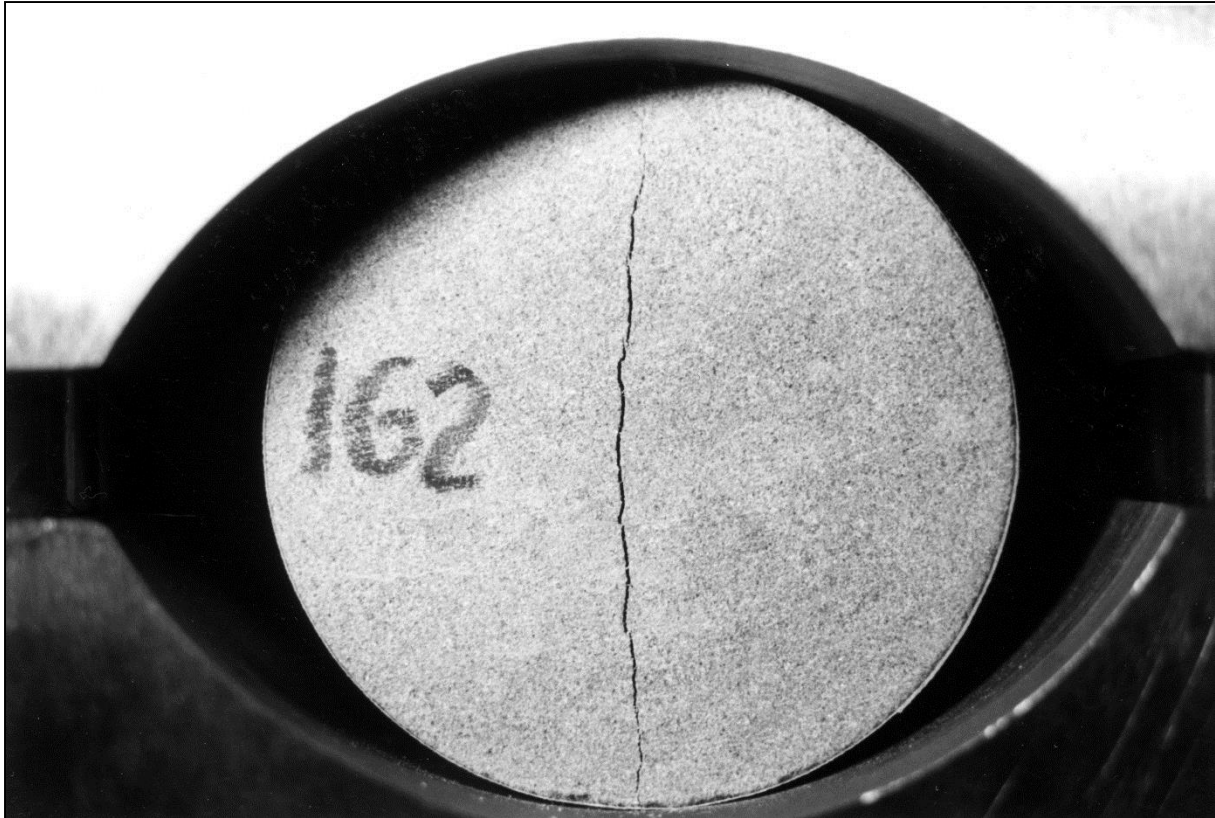
Figure 1-43: A BTS test after failure.
