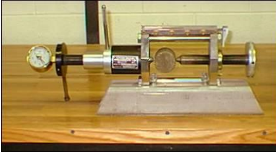
Figure 1-40: Point load test facility (inside.mines.edu).
