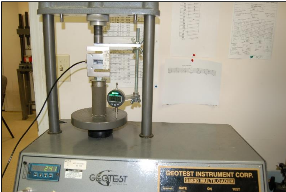
Figure 1-24: A UCS test facility (Timely Engineering Soil Tests, LLC).
