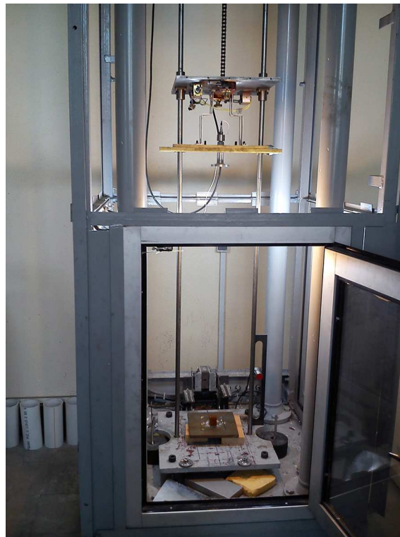
Fig. 2. A copper foam samples in the drop weight testing machine
