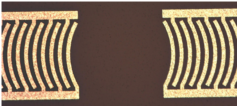
Figure 6.7: Optical image of the SAW device with the 40 0 -arc FIDTs.
