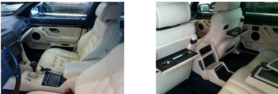
Fig. 20 BMW Individual 7 Series Limousine of the Four Seasons Hotel of Berlin designed by Karl Lagerfeld (BMW Classic) equipped with tables for the rear seat passengers, tissue compartments, an integrated fridge, and a rear seat entertainment system
