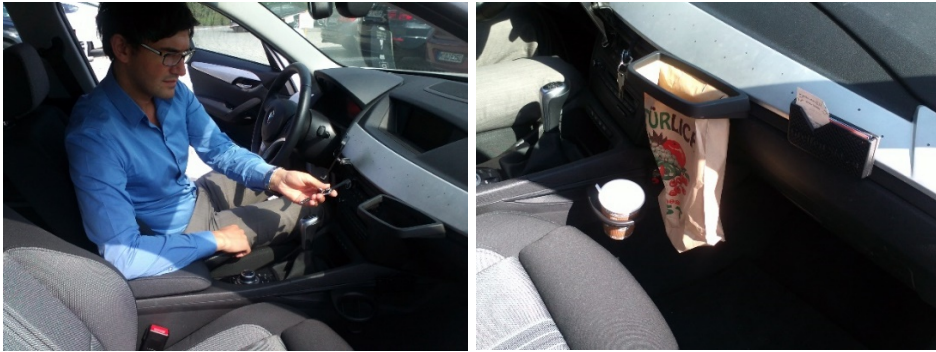
Fig. 22 single-handed use of flexible storage system in mock-up (left), fully equipped version for single person transportation (Ou, Luo, Woodcock, & Wright, 2004)
