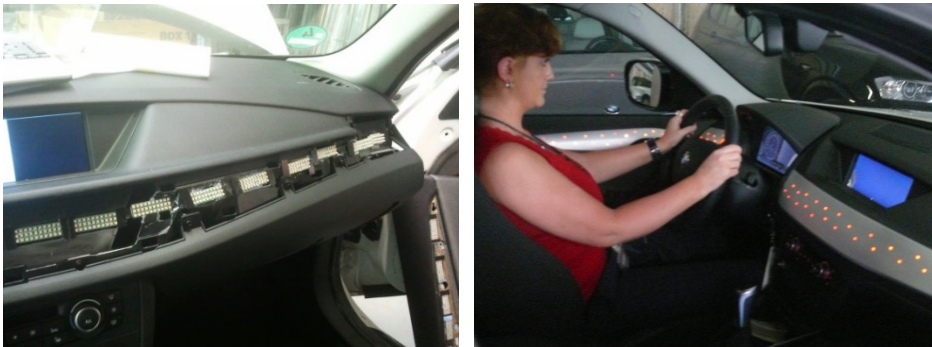
Fig. 32 Adaptive interior lighting mounted in the dashboard (left picture), red lighting of dashboard and door trims adapted to red shirt of driver detected by camera.
