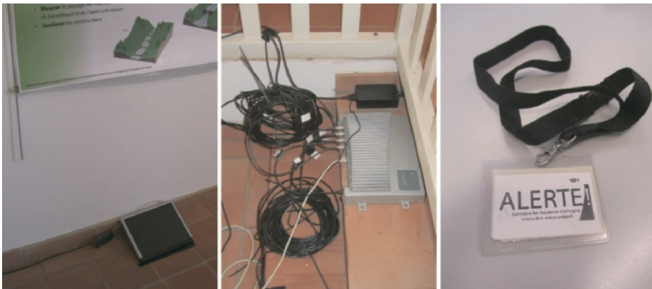
Figure 6.2: RFID appliances from left to right: an antenna, the reader, a passive tag embedded in a badge.
