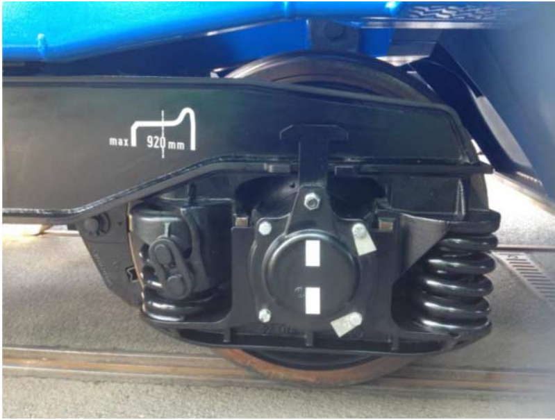
Figure 3. Y-25 primary suspension consisting of a set nested coil springs and a single Lenoir link.
