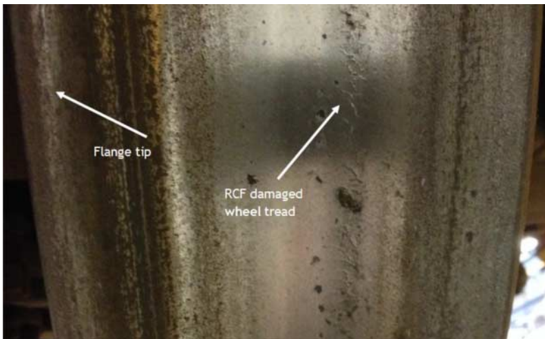
Figure 1. Wheel tread with RCF crack damage.
