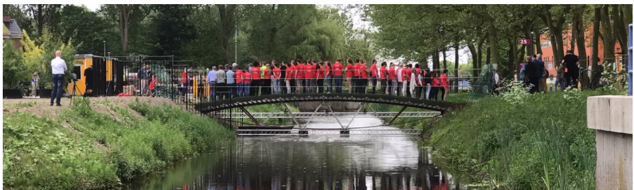
Figure 28 : Load case 1, 67 students, approximately 1.81 kN/m
