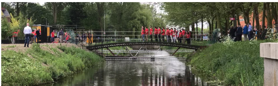
Figure 29: Load case 2, Asymmetric load with 39 students, approximately 2.11 kN/m
