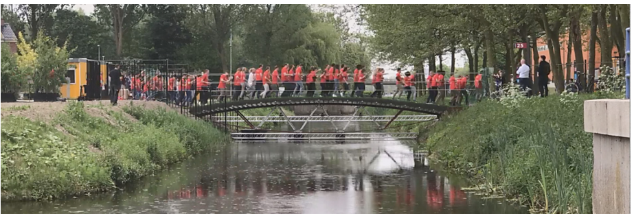
Figure 32: Load case 5, Dancing students, approximately 22.05 kN
