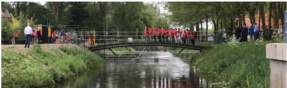
Figure 29: Load case 2, Asymmetric load with 39 students, approximately 2.11 kN/m
