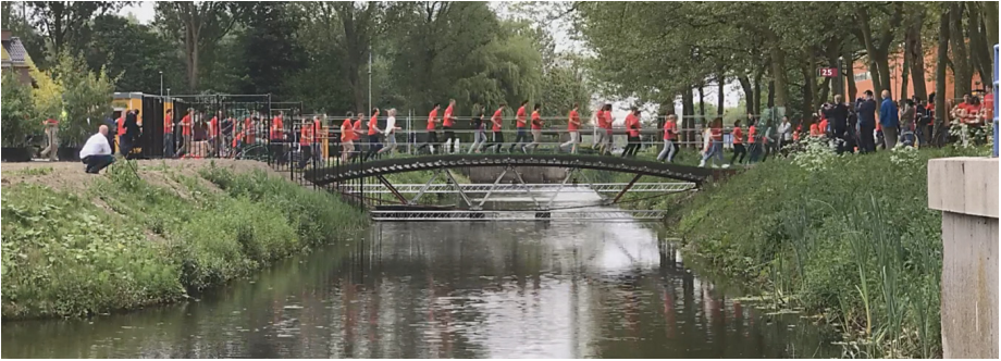
Figure 30: Load case 3, 60 running students, approximately 14.7 kN/m
