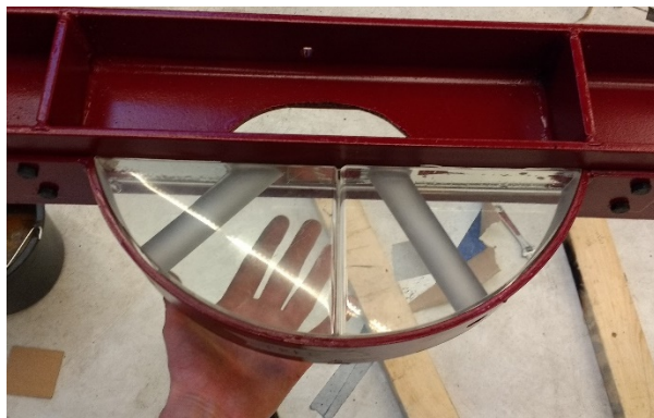
Figure 21: The node after placement in the truss
