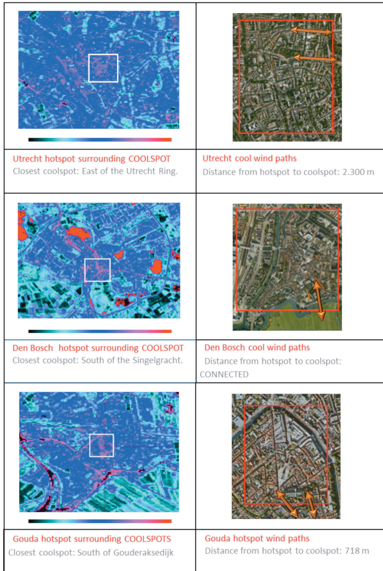
FIGURE 5.12 Coolspot analysis (Storage heat flux map for The Hague, Delft, Leiden, Utrecht, Den Bosch and Gouda 16 July 2006. Landsat image courtesy of the U.S. Geological Survey. USGS/NASA Landsat. further processed with ENVI 4.7 and Atcor 2.3) and wind corridor analysis of the different Dutch cities. Right column google earth imagery.
