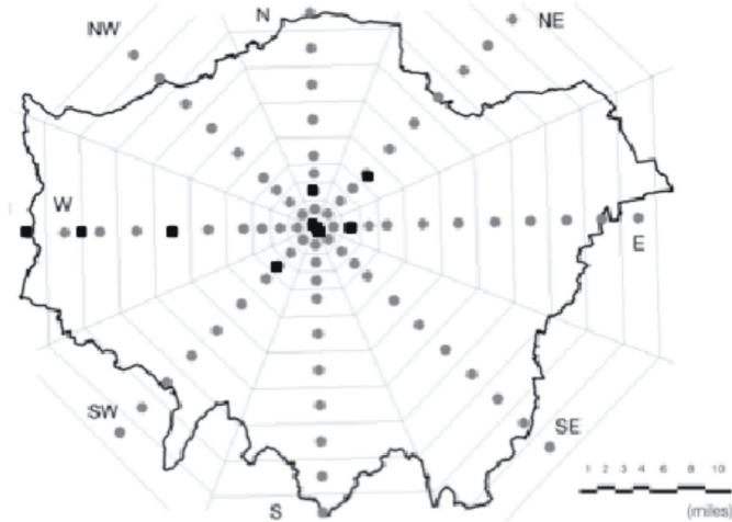
FIGURE 2.11 LSSAT model, fixed temperature stations along the 8 transects of the Greater London Area. Measurement locations are marked in squares.
