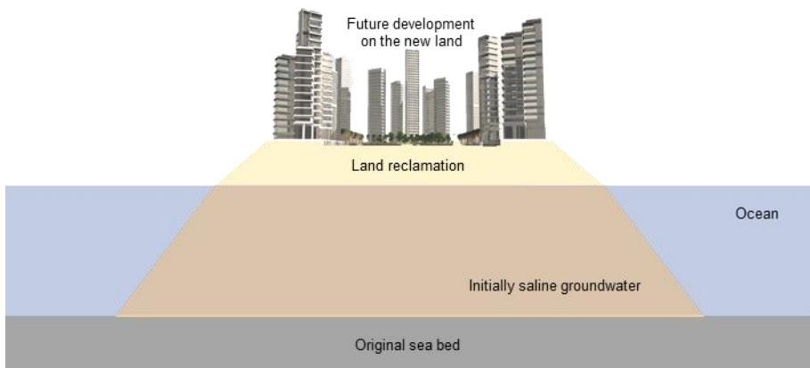
Figure 1: Schematisation of a land reclamation.
