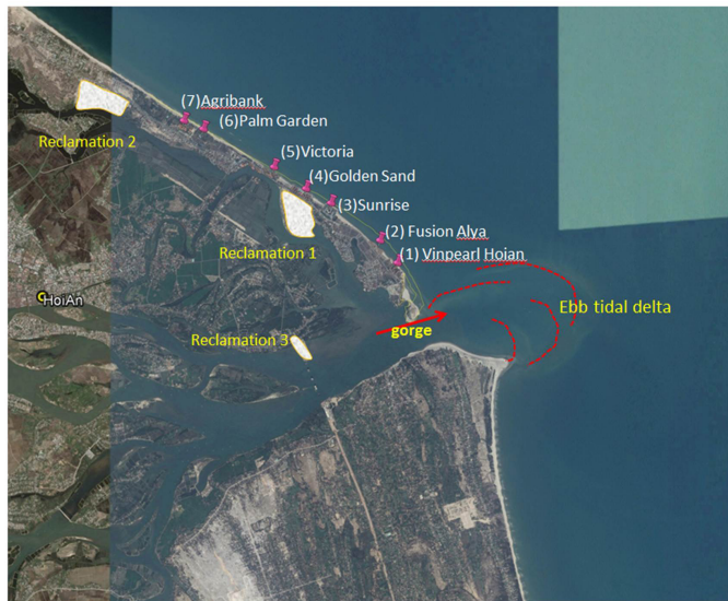
Figure 2.5: Location of resorts and land reclamations and the ebb tidal delta of Cua Dai Beach
